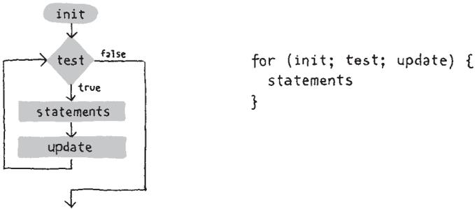
Figure 4-1. Flow diagram of a for loop.
