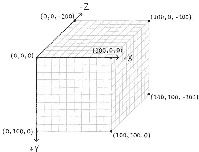
Figure 11-1. Processing's 3D coordinate system.
